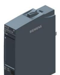
SIMATIC ET 200SP, Signal relay module, RQ CO 4x 24V DC/2A ST, 4 changeover contacts, isolated contacts, packing unit: 1 piece, fits to BU-type A0, Colour Code CC00, substitute value output, module diagnostics for: supply voltage
