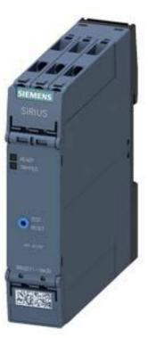
Thermistor motor protection relay Standard evaluation unit 22.5 mm enclosure screw terminal 2 change-over contacts US = 24 V AC/DC Manul/Remote-Reset with ATEX approval 2 LEDs (READY/TRIPPED) galvanic isolation Test/reset button Wire break monitoring Short circuit monitoring
