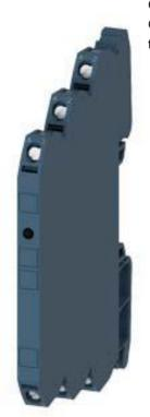
Output coupler Optocoupler 1 NO triac, input 24 V DC Output 20-264 V AC, 2 A Overall width 6.2 mm Screw terminal (push-in) Thermal current 2 A
