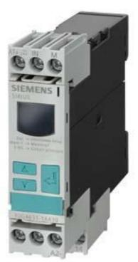
Digital monitoring relay Voltage monitoring, 22.5 mm from 0.1-60 V AC/DC 0vershoot and undershoot 24 to 240 V AC/DC 50 to 60 Hz DC and AC Noise pulses delay 0.1 to 20 s Hysteresis 0.1 to 30 V 1 change-over contact with or without fault buffer screw terminal Successor product for 3UG3531-1AL20, 3UG3531-1AG20
