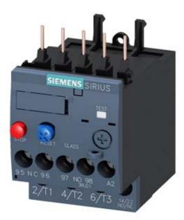
OVERLOAD RELAY 2.2...3.2 A FOR MOTOR PROTECTION SZ S00, CLASS 10, F. MOUNTING ONTO CONTACTOR MAIN CIRCUIT: SCREW TERMINAL AUX. CIRCUIT: SCREW TERMINAL MANUAL-AUTOMATIC-RESET
