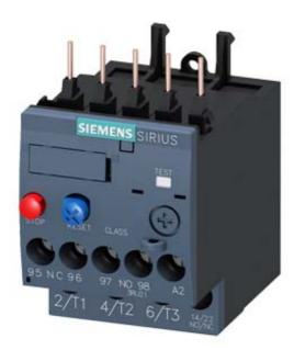
OVERLOAD RELAY 5.5...8.0 A FOR MOTOR PROTECTION SZ S00, CLASS 10, F. MOUNTING ONTO CONTACTOR MAIN CIRCUIT: SCREW TERMINAL AUX. CIRCUIT: SCREW TERMINAL MANUAL-AUTOMATIC-RESET
