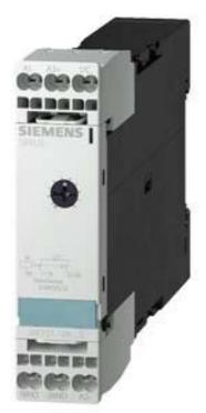
Timing relay, multifunction Phase-out product! For further information, contact our sales department Spring-type terminal 1 NO contact, delayed 1 NO contact instantaneous 1 time range 1...20 s 24 V AC/DC, 200-240 V AC at 50/60 Hz AC
