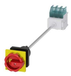
SENTRON, 3LD switch disconnector, EMERGENCY-STOP switch, 3-pole, lu:25 A, Operational power / at AC-23 A at 400 V: 9,5 kW, floor mounting with door coupling, rotary operating mechanism, red/yellow, center mounting 22.5 mm of handle
