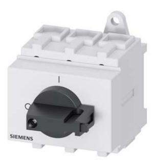
SENTRON, 3LD switch disconnector, main switch, 3- pole, lu:63 A, Operational power / at AC-23 A at 400 V: 22 kW, Distribution board mounting, knob-operated mechanism, black, handle directly on switch
