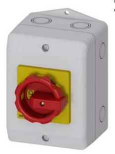
SENTRON, 3LD switch disconnector, EMERGENCY-STOP switch, 4-pole, lu:16 A, Operational power / at AC-23 A at 400 V: 7,5 kW, molded- plastic enclosure for metric threaded joint, 1NC, 1NO, rotary operating mechanism, red/yellow
