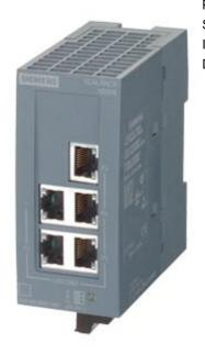
SCALANCE XB005 UNMANAGED INDUSTRIAL ETHERNET SWITCH FOR 10/100MBIT/S; WITH 5 X 10/100MBIT/S TWISTED PAIR- PORTS WITH RJ45-SOCKETS; FOR CONFIGURING SMALL STAR- AND LINE TOPOGRAPHIES; LED-DIAGNOSIS, IP20, 24 V DC POWER SUPPLY, MANUAL AVAILABLE AS **DOWNLOAD**
